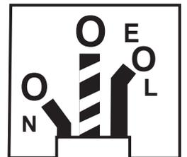
CONNECT GREEN AND - YELLOW WIRE TO PLUG OR SUPPLY TERMINAL MARKED E OR
