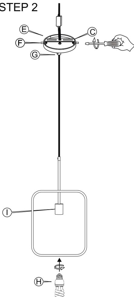
Tighten the canopy (E) with side Screw (F) to the mounting plate (C) and tighten the screw on plastic cord grip (G)
