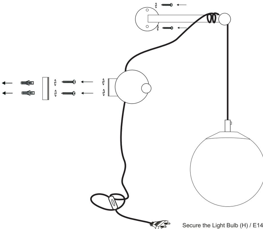
Secure the Light Bulb (H) / E14 into the lamp holder (I).
